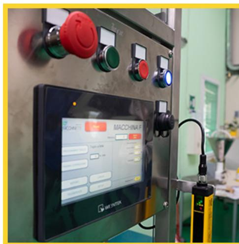
The operating area of the rotary table is protected on three sides by fixed and movable guards. The movable guard is equipped with an electric safety lock, which prevents it from being opened during operation, allowing access only once a complete stop of all electrical and pneumatic movements is guaranteed. In addition, the presence of an emergency stop button (e-stop) allows the cycle to be stopped immediately if necessary.
