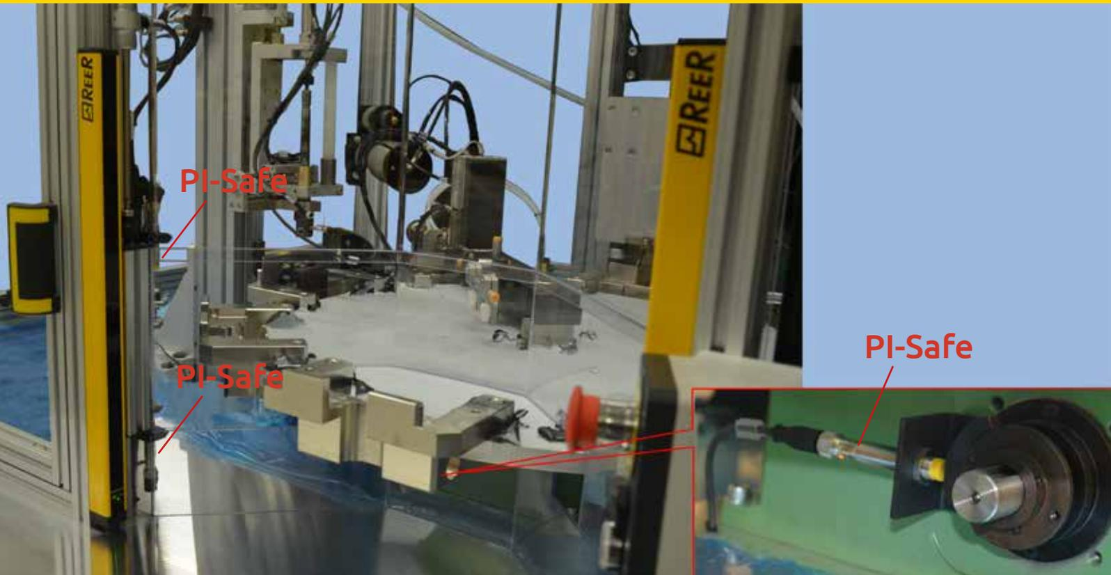
The position monitoring of the protection screen and rotary table are carried out by means of inductive safety sensors PI-Safe M12.
